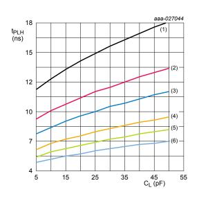
a. HIGH to LOW propagation delay (An to YBn)
