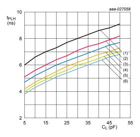
d. LOW to HIGH propagation delay (B4 to YA4)
