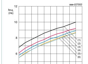
b. LOW to HIGH propagation delay (An to YBn)
